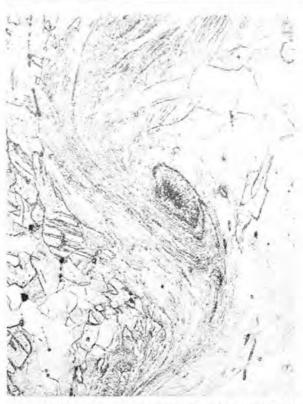
PHOTOMICROGRAPH shows bond region (at 400X magnification) between copper plates produced by impact welding technique.
